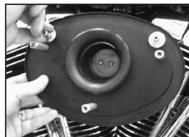
12. Reinstall the back plate and thread the stock breather bolts into the breather bolt extensions. Do not tighten at this time. Note: For 2006-2007 fuel injected models, reinstall a washer in between the back plate and each of the provided breather bolt extensions. Thread the stock breather bolts into the breather bolt extensions. There should be a washer on each side of the provided breather bolt.
