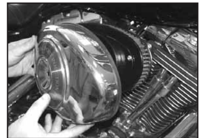
20. Reinstall the stock air cleaner cover and completely tighten.
