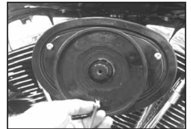
17. Reinstall the three button socket bolts. (Reuse the button head bolts removed from step 2) Do not completely tighten.
